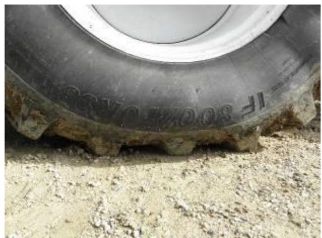
**High flexing 372 AGRIFLEX increases contact area significantly and thus reduces ground pressure.**
