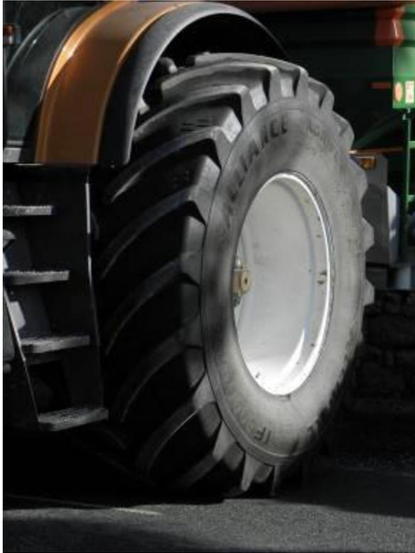
372 AGRIFLEX is a large volume Improved Flexion tyre designed for use in High HP tractors (Like the 250HP Renault of the Duprezs') and combine harvesters. The tyres are rated at 'D' speed rating and can be driven at speeds up to 65kph on road. This radial tyre is steel belted, which provides even ground pressure and superior resistance to punctures.
