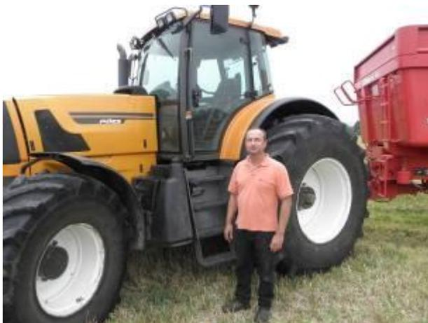
In June 2014, they equipped one of their Renault Atles 936 RZ with Alliance 372 AGRIFLEX the Improved Flexion technology tyre. The tractor was earlier shod with Goodyear rubber. The sizes are IF 800/70R38 184A8 CFO 372 AGRIFLEX (Rear) & IF 600/70R28 164D 372 AGRIFLEX (Front). Since then the tyres have completed more than 800 hours in the tractor. The rear tyres run on an air pressure of 1.3bar and the front tyres with 1.2bar.
