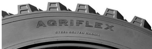
The AGRIFLEX patterns are steel belted radial tires, designed to carry 20% more load with standard air pressure, or carry a standard load with 20% lower air pressure. The lower air pressure along with high flexing sidewall increases the tire's footprint area significantly, reducing ground pressure.
